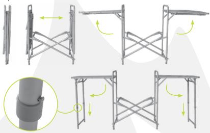
2. Ensure the corner locking brackets are firmly in place.
